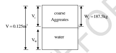
$Volume(V) = V_{C} + V_{w}$
