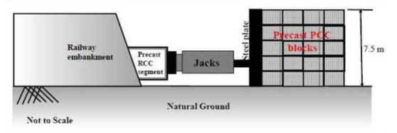
At each stage, the jacks are required to apply a force of 1875 kN to push the segment. The jacks will react against the rigid steel plate placed against the reaction arrangement. The footprint area of reaction arrangement on natural ground is 37.5 m<sup>2</sup>. The unit weight of PCC block is 24 kN/m<sup>3</sup>. The properties of the natural ground are:  $c = 17 \text{ kPa} \phi = 25^{\circ}$  and  $\gamma = 18 \text{ kN/m^3}$ .
