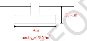
As per Terzaghi's theory, For square footing Ultimate bearing capacity  $(q_u) = 1.3 \text{CN}_{\text{C}} + \gamma \text{D.N}_{\text{q}} + 0.4 \gamma \text{B.N}_{\gamma}$
